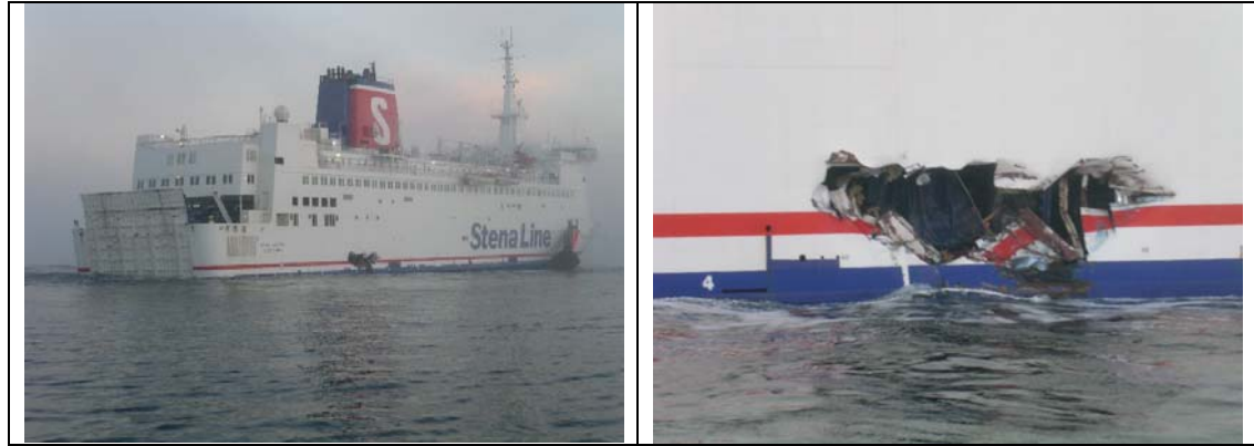
The upper part of the damage in to the cargo deck
