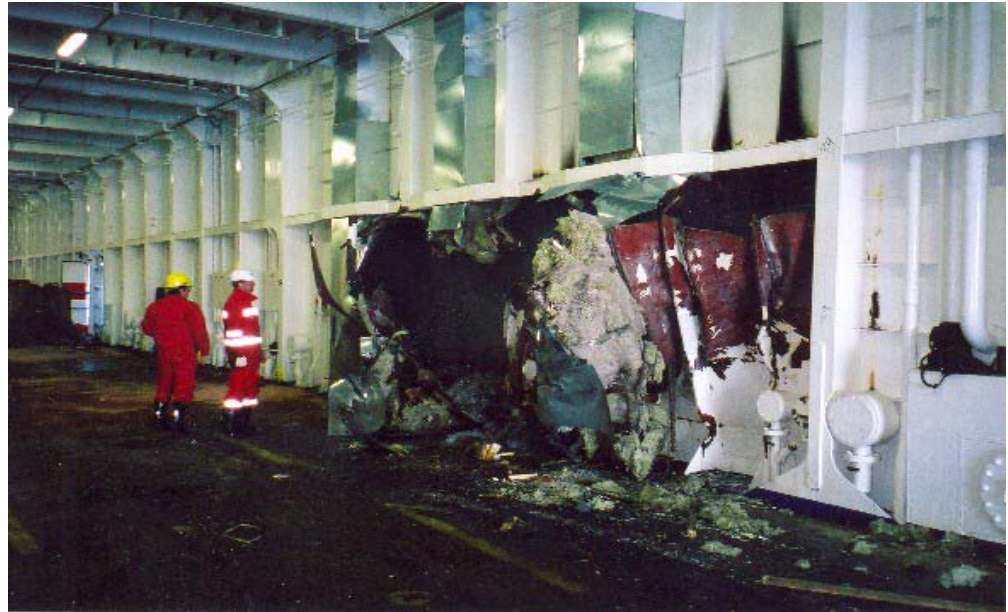
The damage in Stena Nautica seen from the cargodeck
