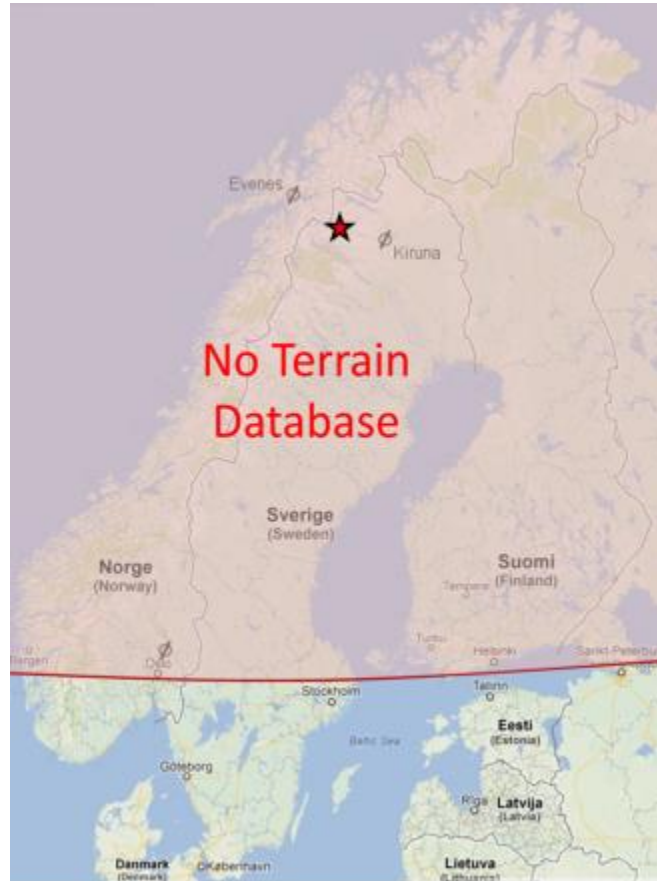
Fig. 10. Map of Scandinavia. In the red area, TAWS in Tactical mode has no terrain warning function. The crash site is marked with a red star (Map view from Google Maps)
