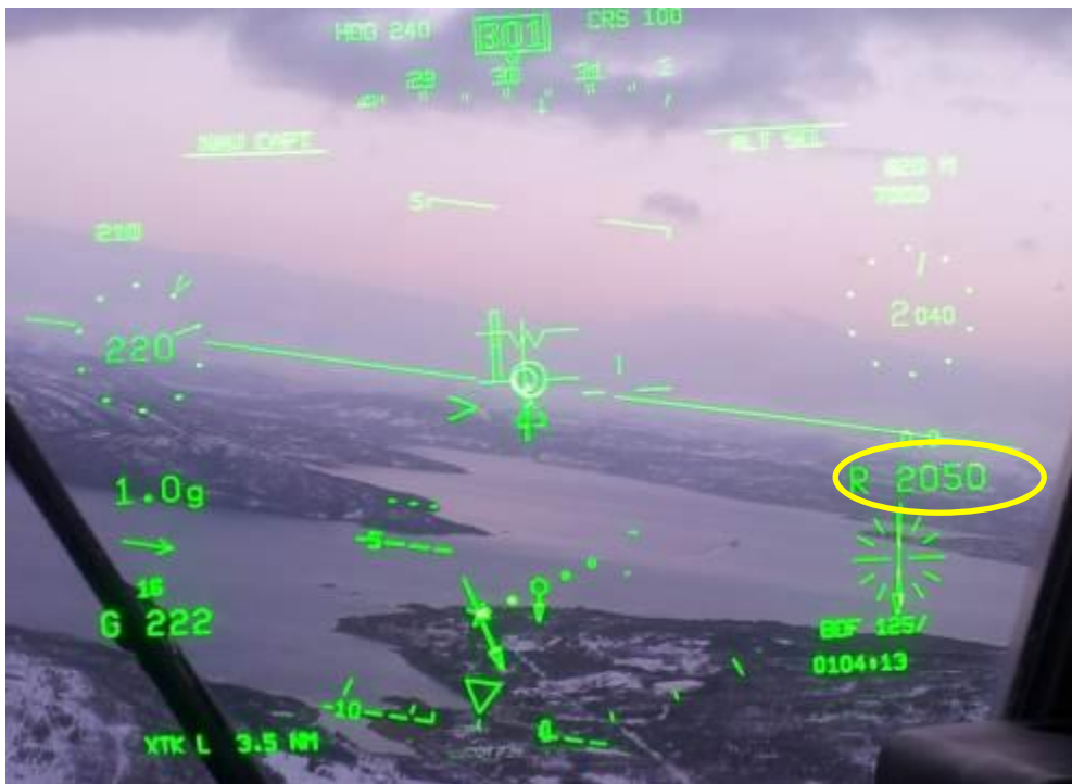
Fig. 9. Picture of the Head Up Display, HUD, with the current radar altitude circled in yellow. (Picture: Norwegian Air Force)
