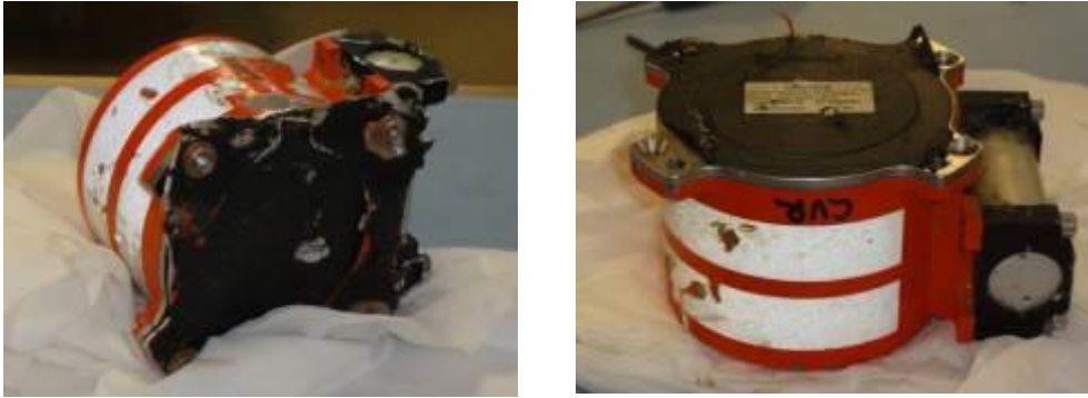
Fig. 23-24. The crash-protected memory units from DFDR and CVR. (Image SHK.)
