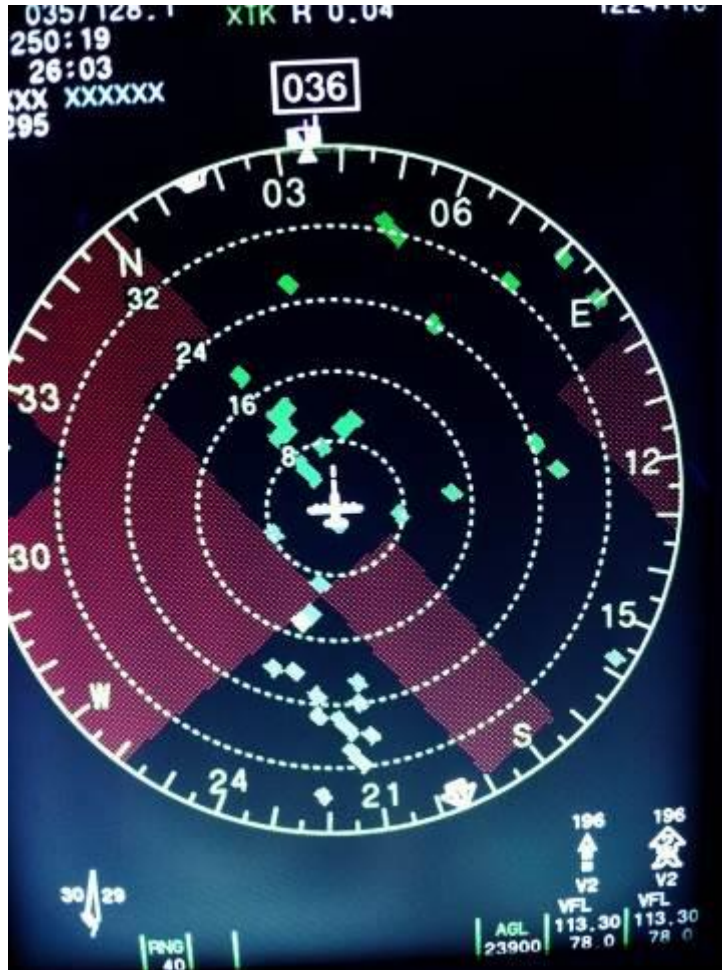
Fig. 11. Photo of the TAWS display at a position north of 60° N. Areas with “voids” appear in magenta. The green dots show obstacles. When flying in black areas, the VOID message is off. (Picture: Norwegian Air Force)
