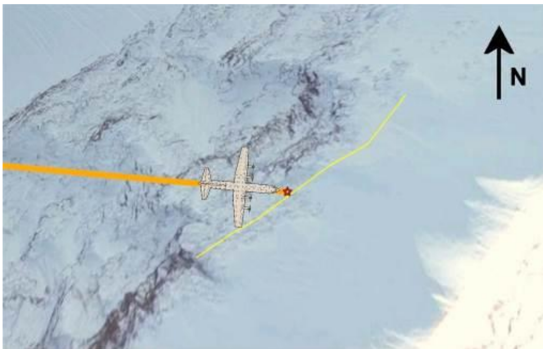
Fig. 27. Photo montage of the point of impact, as seen from above. The contour line at the point of impact is marked with a yellow line, and the aircraft's approach with a thick orange line. (The picture is based on a satellite image from Google Earth.)
