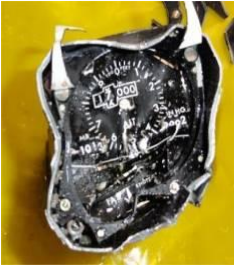
Fig. 35. Standby instrument for altitude and airspeed. (Photo: SHK)
