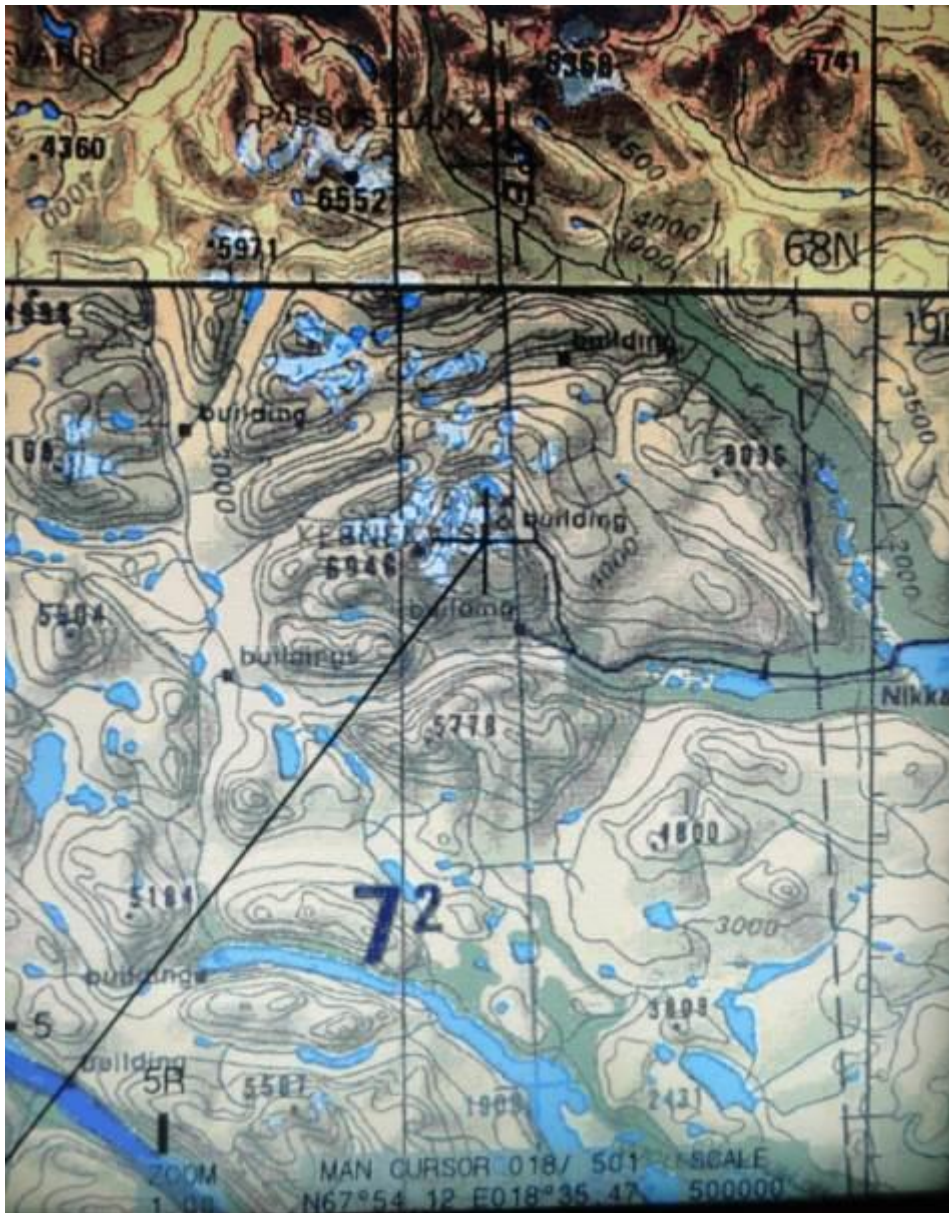
Fig. 14. Moving map. However, the cursor line and the scale are misleading in relation to the sequence of events. (Photo: Norwegian Air Force.)
