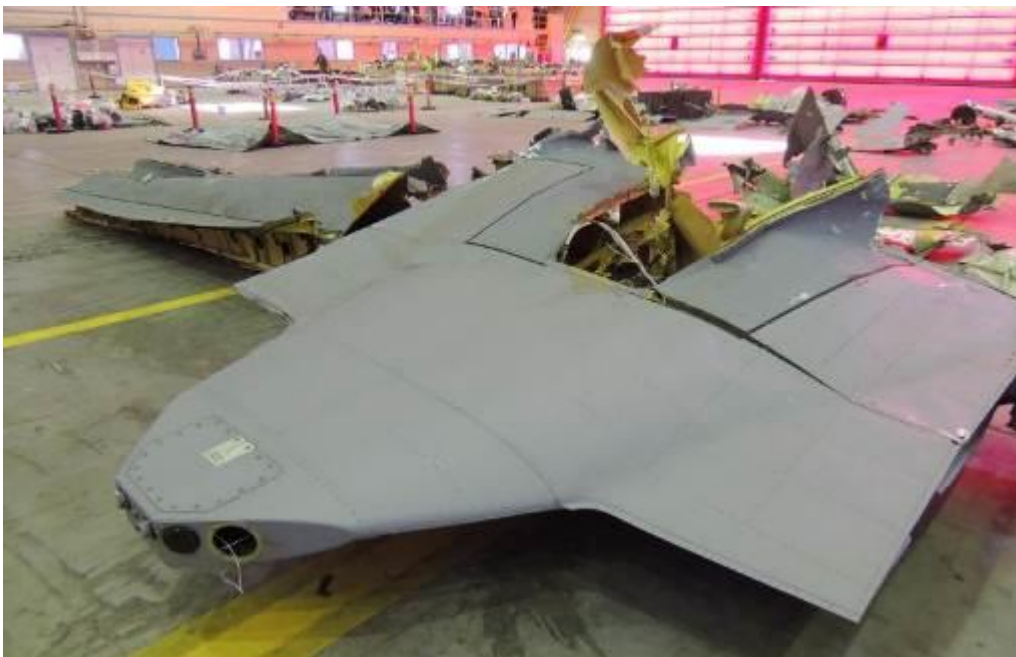
Fig. 30. Some of the larger parts of the wreckage in the hangar. Parts of the tail section in the foreground. (Photo: SHK.)
