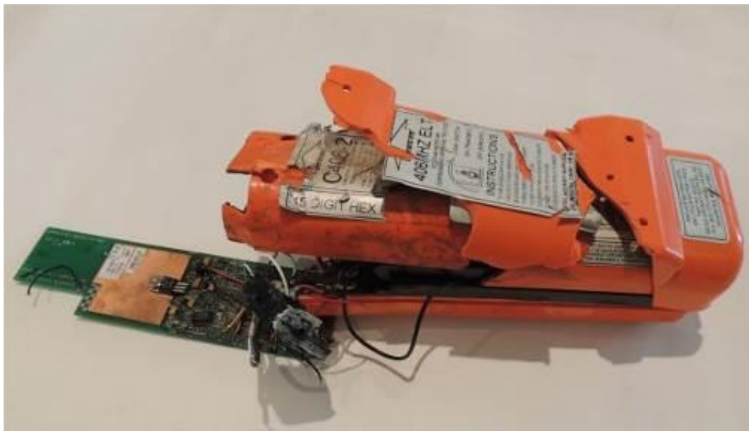
Fig. 31. Photo of the aircraft's ELT, Emergency Locator Transmitter. The damage to the unit is greatest in the forward part, on the left of the picture, where the antenna connection is located. (Photo: SHK)
