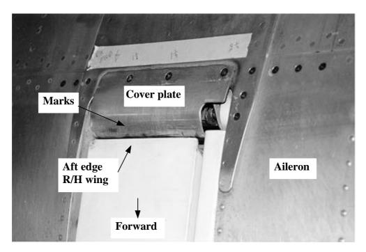
All corresponding cover plates in question in the company's fleet were inspected. It was found that the screws were tightened but that the play at the aft edge of the wing varied between 0.0 and 2.0 mm.
