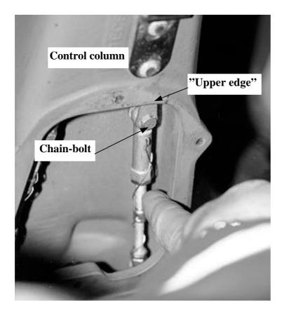
The left control column as well as all other control columns of the airline's other aircraft proved when checked also to have chains that were more or less slack.
