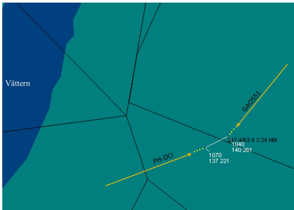
Fig. 1. Radar tracks with the minimum vertical distance of 300 feet at a horizontal distance of 3.24 nm.
