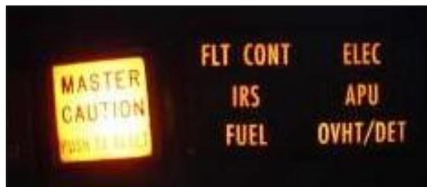
Fig. 3. Warning and annunciator panel on the glareshield in front of the left seat.
