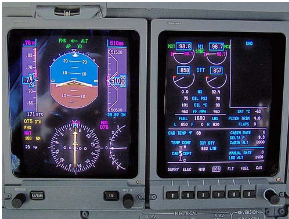
Fig. 11. The PFID is displayed to the left and the MFD to the right.
