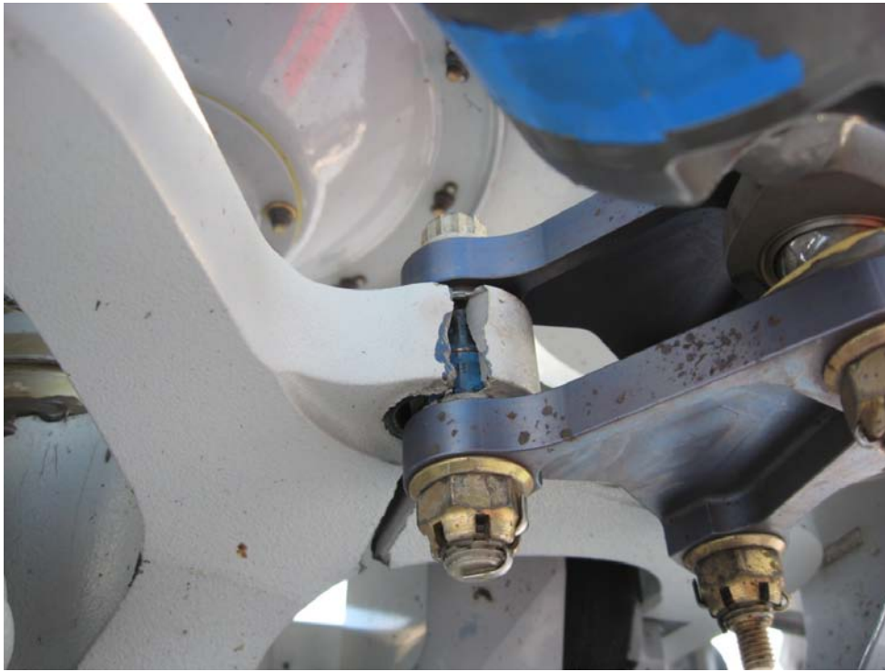
Fig. 7 The main rotor hub with a visible crack.
