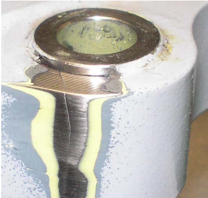
Fig. 10 Ear on the damaged rotor hub with exposed crack, item S/N 1070.
