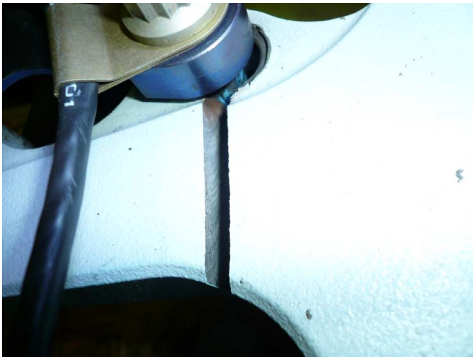
Fig. 8 Main rotor hub with fatigue crack, as seen from above.
