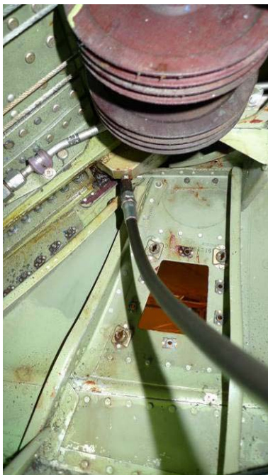
Fig. 9 Lubrication of stabilizer hinges via panel 6309A
