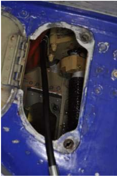
Fig. 8, Lubrication of the stabilizer jack screw support assembly via panel 3701A
