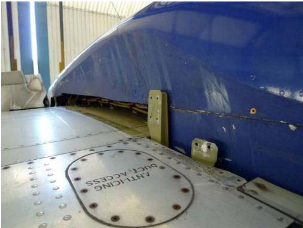
Fig. 1 The area where panel number 3806A should have been mounted, looking backwards
