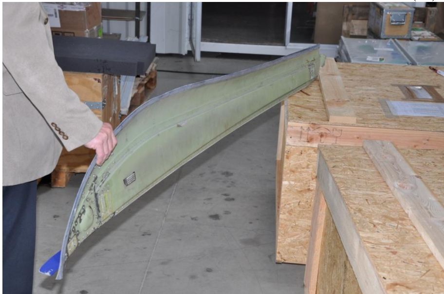
Photo 12: The rear of the fairing is in line with the wooden strip, this illustrates a bend in the fairing of approximately 60deg.
