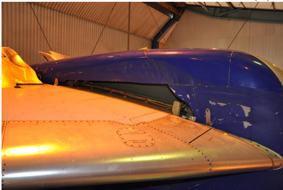
Photo 1: Area of RH horizontal stabilizer showing missing upper fairing.
