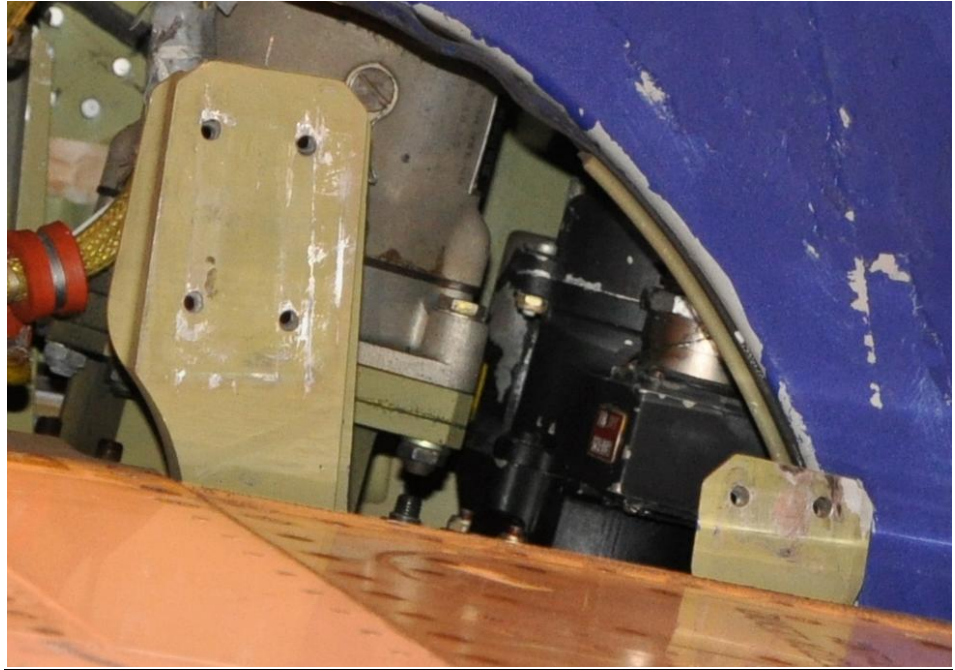
Photo 5: Mounting brackets for 2-NAS1203-4 & 2-NAS1203-11 + 2-NAS1203-10, RH horizontal stabilizer.
