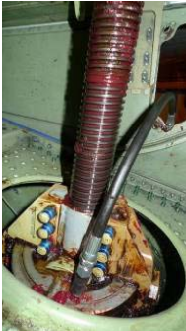
Fig. 7 Lubrication of stabilizer jack screw gimbal ring via panel 3701A
