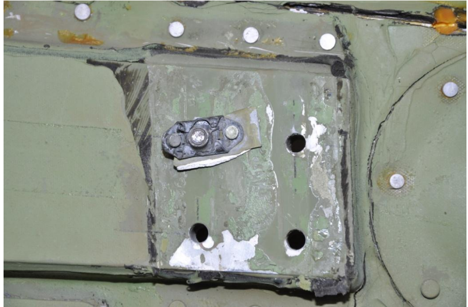
Photo 7: Internal view of the fairing showing the remaining screw, fastener and attached failed piece of bracket.
