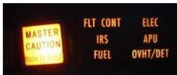
Fig. 3. Warning and annunciator panel on the instrument panel in front of the left pilot.
