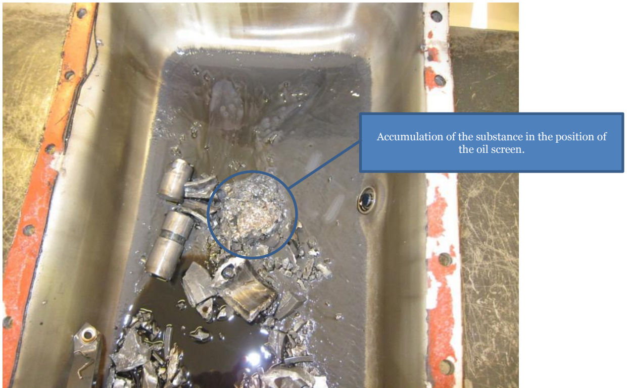
Figure 9. Deposits and remnants of engine parts in the oil pan.
