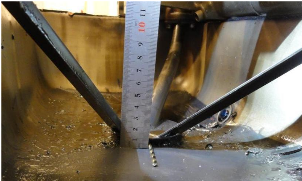
Figure 7. Position of the oil filter. Note that the oil drain is positioned at the side, roughly 15 mm above the bottom of the pan. The drill bit in the image serves as a dimension reference and has a diameter of 3.5 mm.
