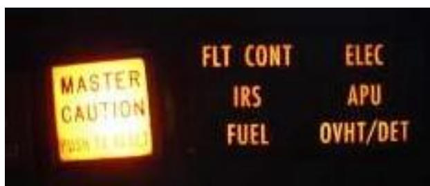
Fig. 3. Master caution system panel on the instrument panel in front of the left pilot. (Photo: SHK)
