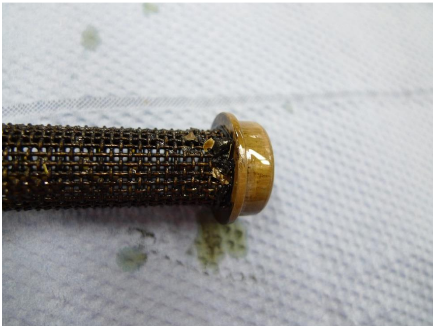
Fig. 5 The main transmission's coarse screen meshing with contaminants of sealant and paint debris.
