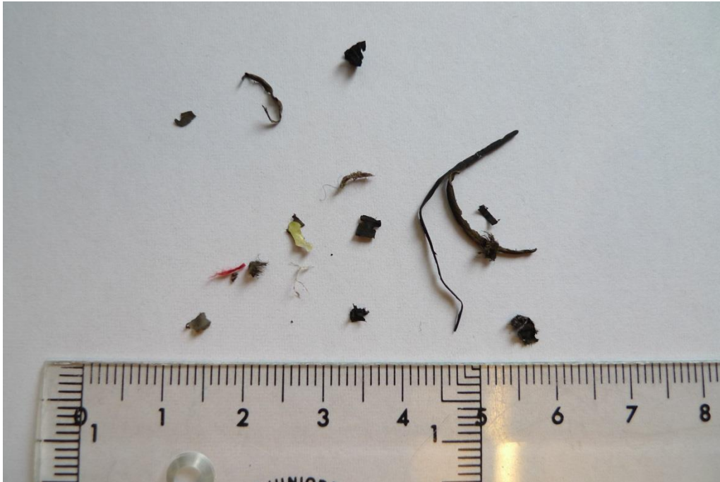
Fig. 4 Contaminants from the filter housing (screen filter) on the main transmission, debris from o-rings, sealants, textiles and paint.
