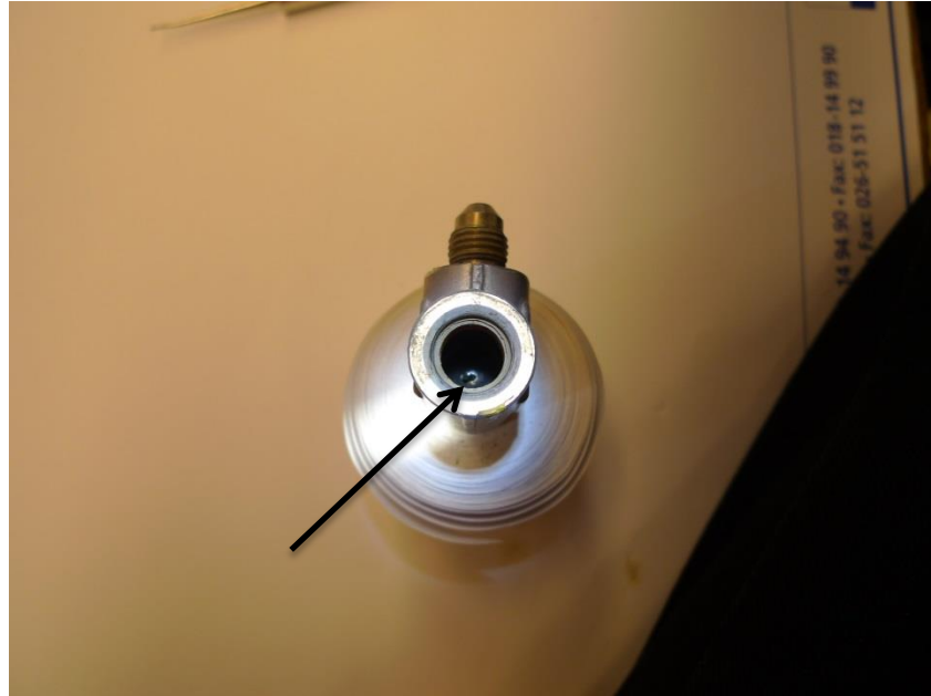
Fig. 6 Restrictor P/N 206-040-244-001, the contaminant is visible at the arrow tip.
