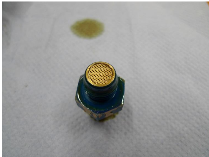
Fig. 10 Filter P/N 50-075-1. Upon examination, the filter was free from visual contaminants.
