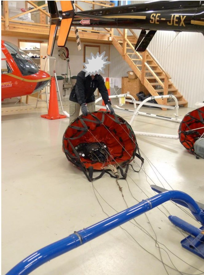
Figure 10. Bambi Bucket angled about 30° to the left behind the helicopter.
