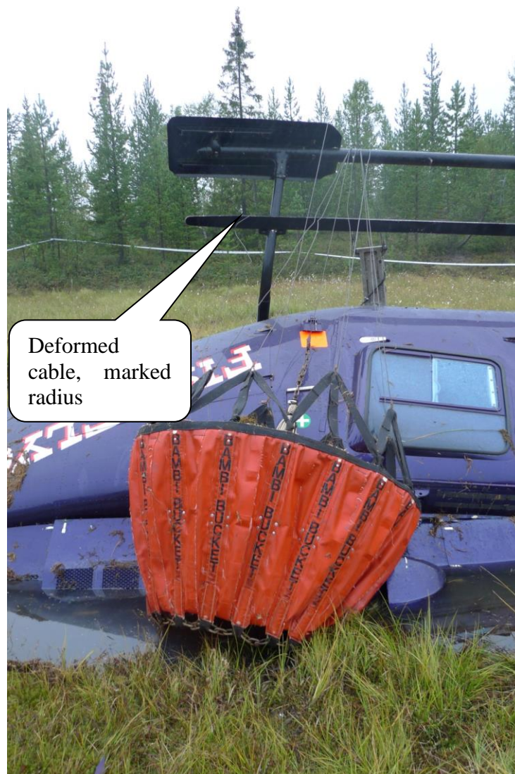
Figure 6. Bambi Bucket, left skid and skid shoe, note the radius of the marked cable.
