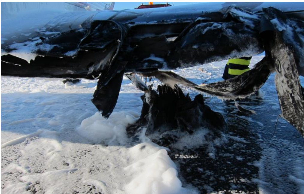
Fig. 3. Damage to wheel, wing and flap. Photo: Borlänge Rescue Services.
