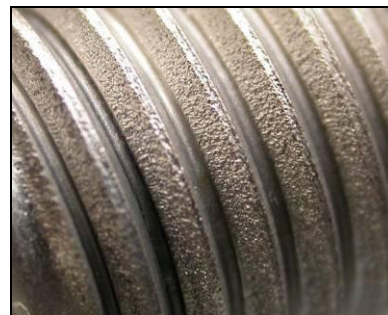
Figure 13. Worn securing threads
