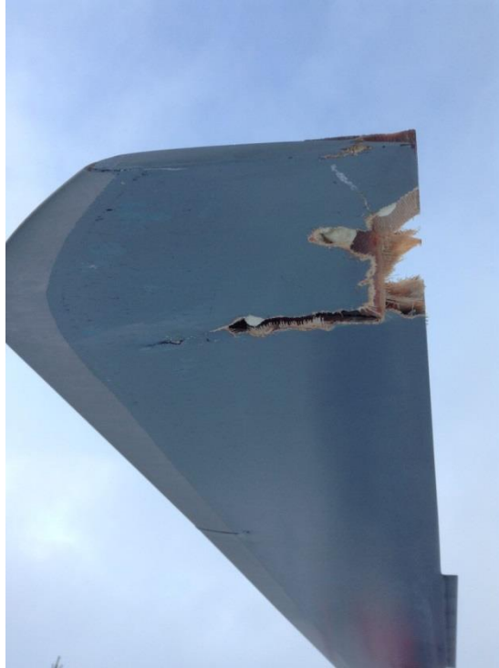
Figure 6. The image shows the rotor blade that sustained the most damage. Source: Jämtlandsflyg AB.
