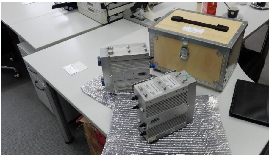
Figure 4. Examination of the FADEC units in Hamburg.
