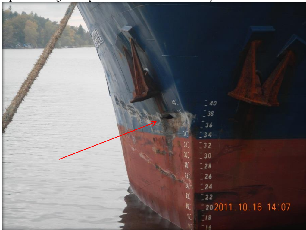
Fig. 6. Damage to the Liva Greta.
