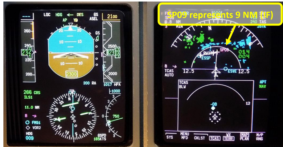
Figure 9. Picture taken from the simulator of left pilots PFD and MDF with a range of 25 NM.
