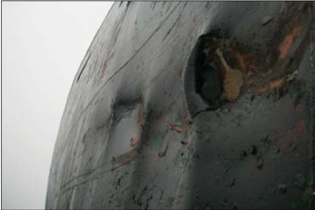
Figure 3: Breached hull above the vessel's water line
