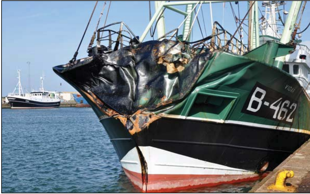
Figure 8: Damage to Vidar 's stem as seen from the port side
