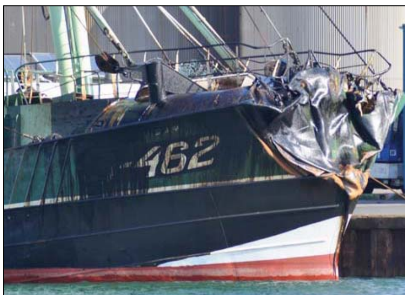
Figure 7: Damage to Vidar 's stem as seen from the starboard side
