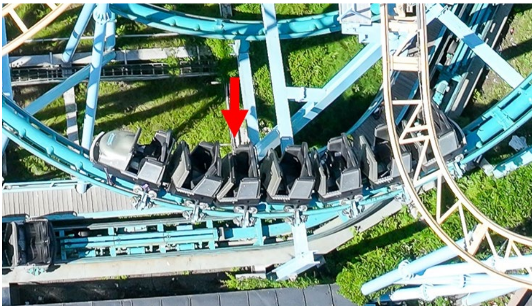
Figure 14. Picture of the train following the accident. Note that the front of car three has bent backwards (marked with an arrow).
