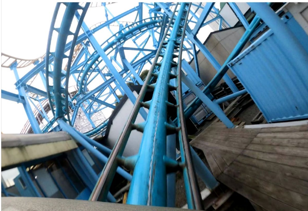
Figure 23. Picture from the test run that shows the train in the position of the first impact on the track. At this time, the speed was 88 km/h and the load was 4.7 g in the front car.
