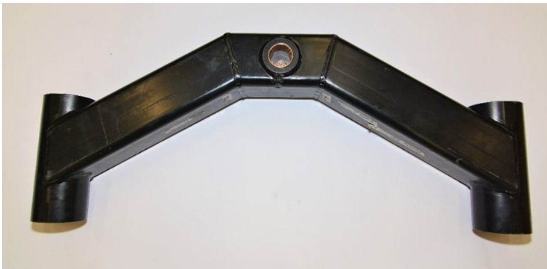
Figure 8. A front control arm on a Jetline train with the hole in the middle for the axle attachment to the car.
