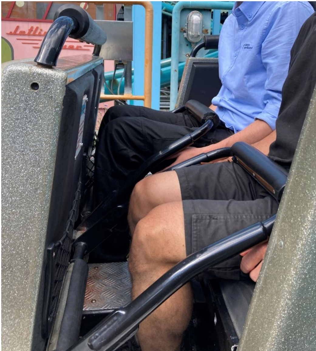
Figure 9. The lap bars in the cars that were lowered against the stomach/thighs.
