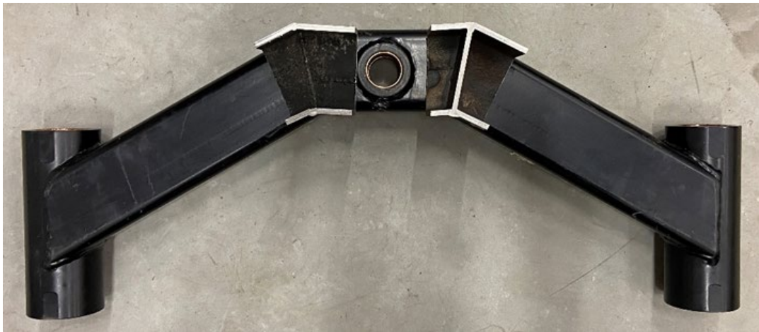
Figure 19. The picture shows a control arm with cut-out samples laid on top. The sample on the left is from a control arm manufactured in 2019 and the one on the right is from an original control arm. The transverse metal plate that is absent on the left is visible in the section on the right.
