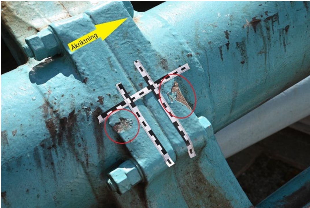
Figure 11. The first impact mark on the track. The red markings drawn in by SHK show where the impact occurred and the yellow arrow indicates the direction of travel. The black and white tape markings were added by the Swedish Police Authority.
