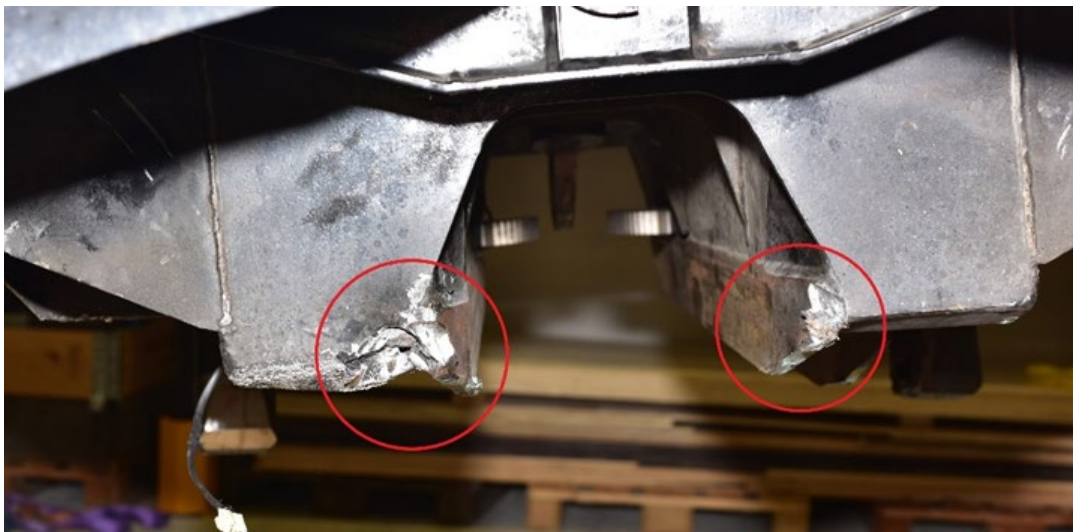
Figure 13. Damage to the underside of the front car. The red markings show where the impacts occurred.
