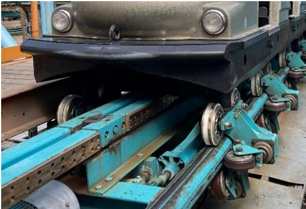
Figure 2. The front part of the train with the bogies with wheels above, under and on the sides of the rail. (The picture does not depict the train involved in the accident.)
