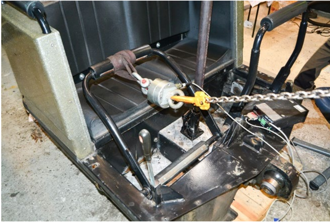
Figure 22. Rigging used during load tests on a lap bar.
