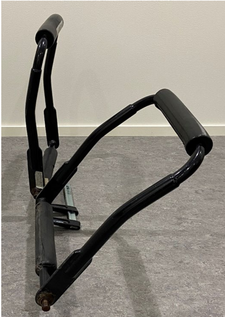
Figure 21. The lap bar from car 5, left, has been placed behind an undamaged bar. The bar from car 5 was bent forward c. 30 degrees to an almost open position during the accident.
