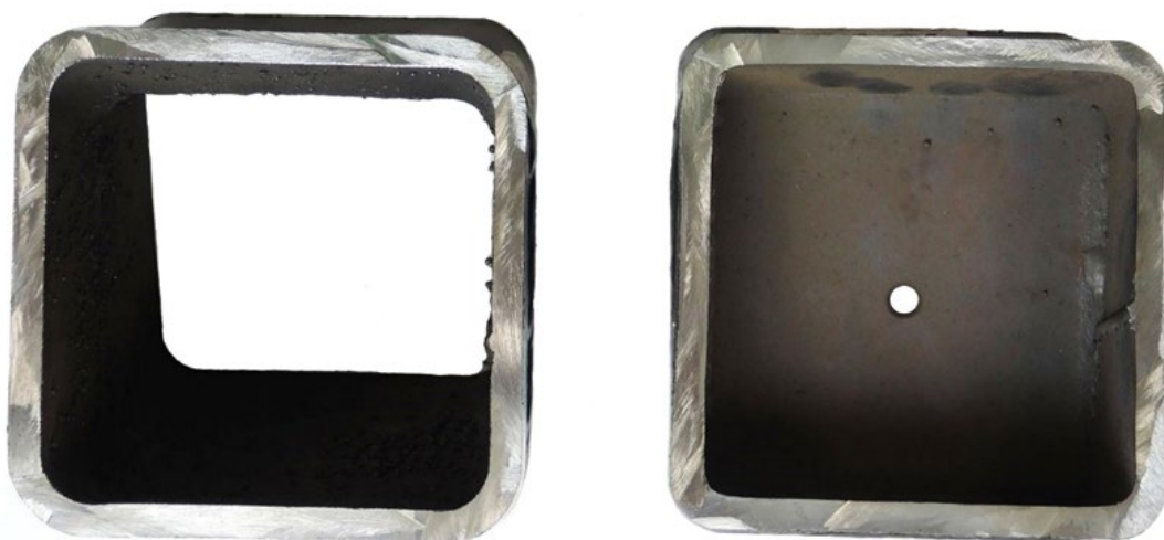
Figure 18. Cross-sections of two cut-up control arms. Original control arm manufactured in 1986/87 on the right and control arm manufactured in 2019 on the left. Image: Element Materials Technology AB.
