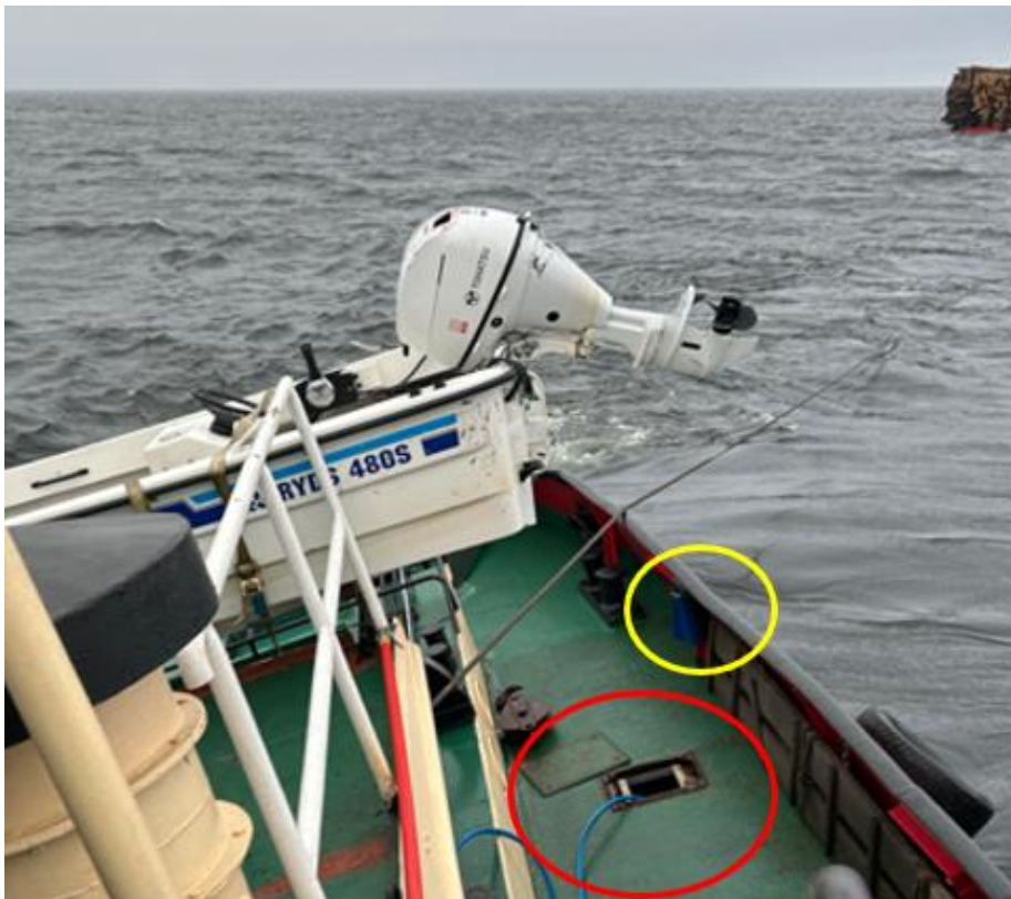
Figure 5. The red marking shows the open manhole to the port ballast tank, where a blue pump hose is inserted. The yellow marking shows the gooseneck for the same tank. In the upper right corner, the barge can be seen, connected to the vessel by the towing wire running out over the port rail. Photo taken by the crew at 04:47. Image: The Shipping company. Annotations added by SHK.
