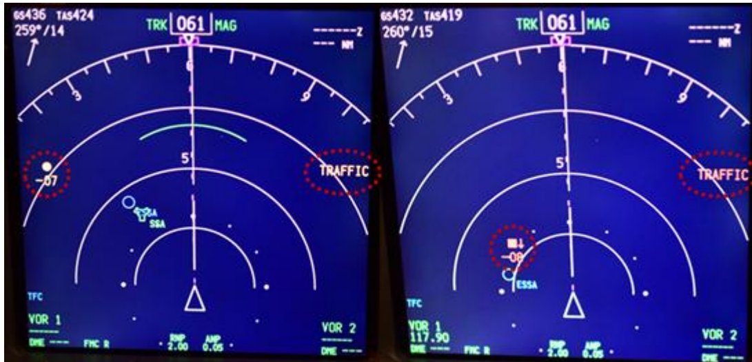
Figure 4. On the left, the Navigation Display is shown during a TCAS TA, and on the right, the Navigation Display is shown during a TCAS RA. The symbols are marked by the SHK with a red dashed circle.
