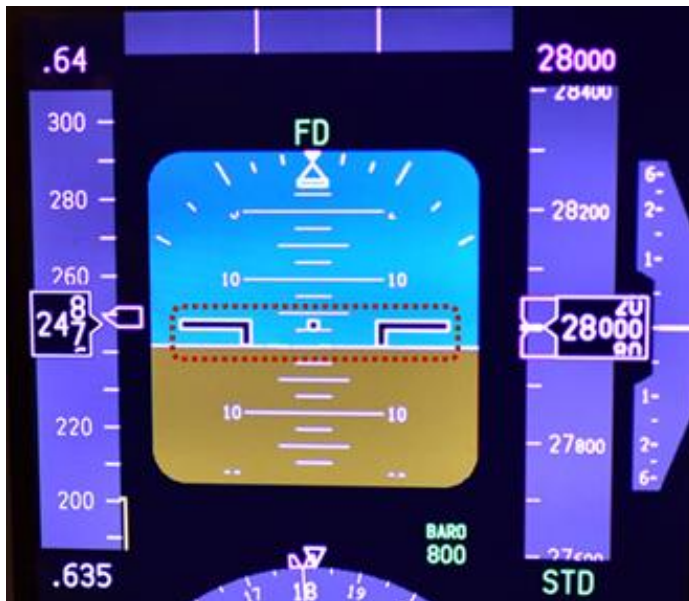
Figure 5. PFD with the aircraft symbol marked by SHK with a red dashed line.
