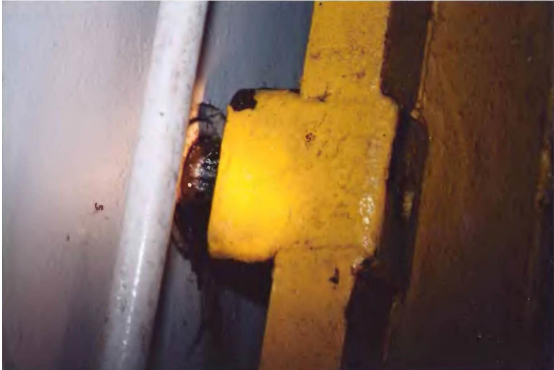
Fig. 3.6. The picture shows bow ramp lower locking, seen from car deck. The locking itself is inside the wing house (on the other side of the white painted hull). When locked, the locking pin is hydraulically pushed (to the right in the picture) into the yellow housing and to unlock, the locking pin is to be hydraulically pulled out (to the left). This shows that it is not possible to hit the locking from car deck. However, it would be possible to hit the yellow housing into which the locking pin is to be pushed or pulled, having the vibrations to facilitate the movement of the locking pin. The picture is from the vessel MARE BALTICUM. Compare to Fig. 3.3 above.
