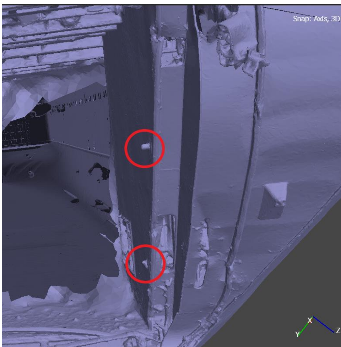
Fig. 3.1. The picture is from photogrammetry in 2022 and shows the both bow-ramp lockings on port side, hull part. The lower is not in fully extended position. A diver estimated in 1994 the degree of extension to "1.5 inches" (some 3 cm) instead of the full length, about 15 cm. If this was the circumstance when leaving Tallinn, a green light would not have shown on the indication panel at departure.
