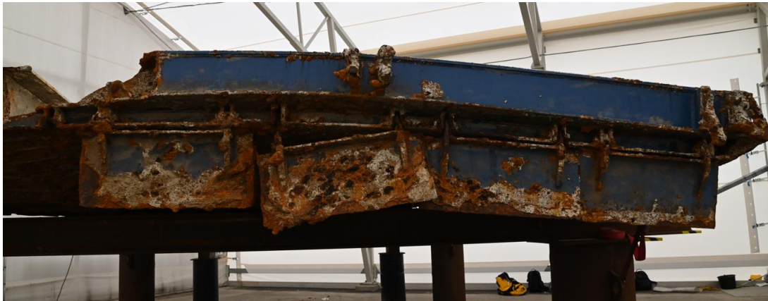
Fig. 3.5. The car deck bow ramp, port side to the right (the ramp is up-side-down on the picture). Four flaps are still connected to the ramp, hanging in their hinges. The picture is cropped.
