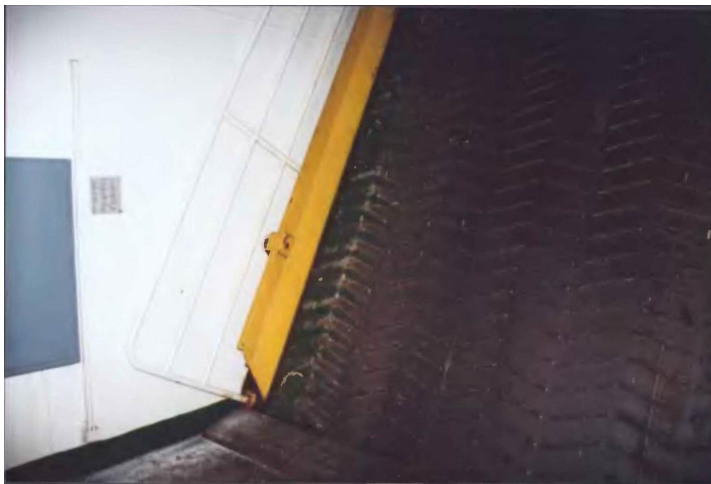
Fig. 3.3. As can be seen from this picture, there is a built-up edge at the side of the ramp, coming close to the bulkhead. Above the edge, the ramp railing hinders access to the area between edge and hull. At the bottom of the ramp, a flap can be seen. The flaps may be folded up to reach the area below for maintenance. The picture is from the vessel MARE BALTICUM, which was constructed in the same way as MV ESTONIA.
