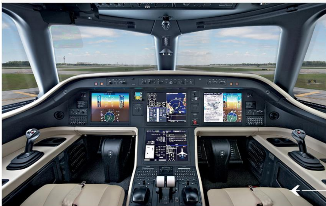
Figure 1. Design of the Cockpit. Screens display flight instruments and system information. Image: Embraer.
