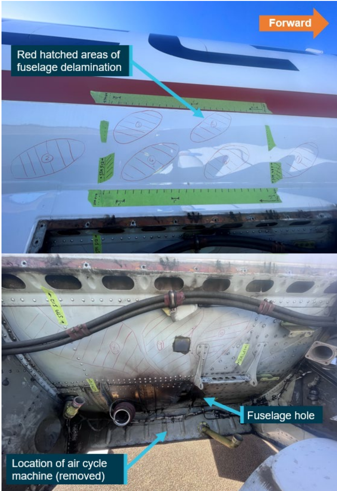
Figure 10: Right side delamination on fuselage
