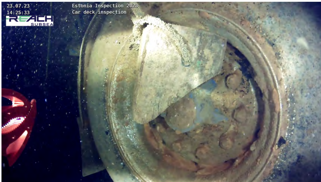
FIG. 5.3: Footage from the car deck shows a cargo securing chock next to the shifted cargo unit on the car deck of MV ESTONIA during the visual inspection in 2023 (O 2.21).
