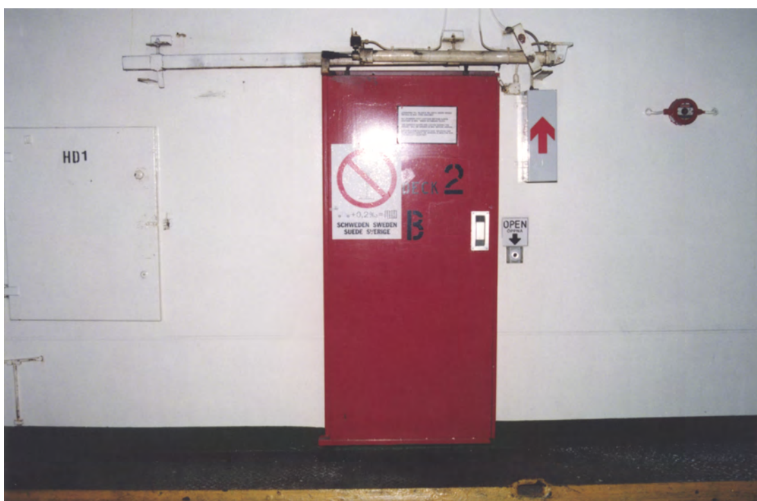
FIG. 4.7: Sliding fire door on the car deck of MV MARE BALTICUM, the near-sistership of MV ESTONIA. Source: Börje Stenström, 1995-11-07, SHK Archives, F 1 HB. 23A B15.6.
