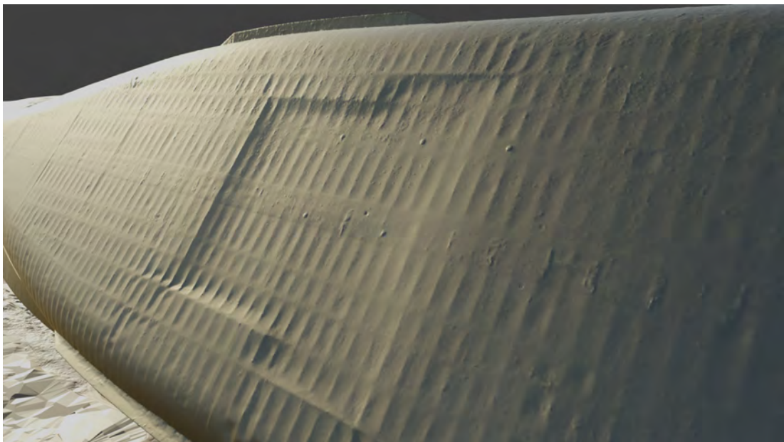
FIG. 3.44: Buckling of the flat bottom
