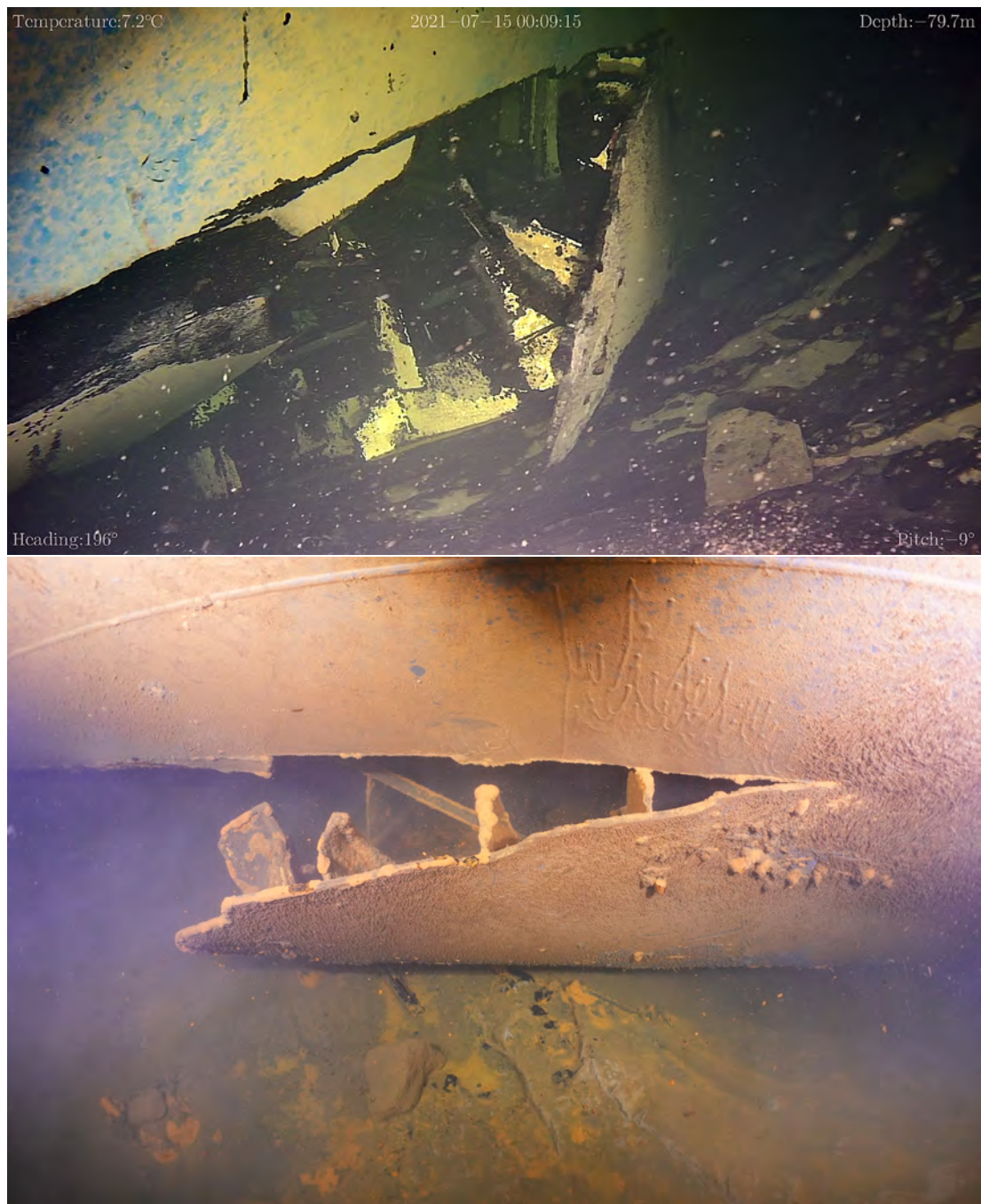
FIG. 3.37: Starboard side aftward penetrating damage close-up. Upper image is from 2021 ( O 2.13 ), the lower from 2022 ( O 2.20 ).
