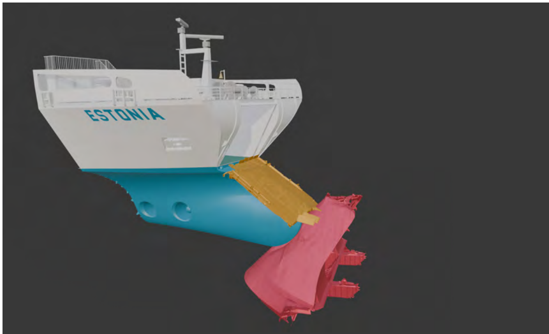
FIG. 4.5: Physical damage of the bow visor and the ramp confirming the full opening of the vessel's bow entrance at the beginning of the accident. The large dent in the front side of the visor (red) is aligned with the bulbous bow and the ramp's (yellow) underside deformations are aligned with the forepeak deck. Visor actuators are not shown.
