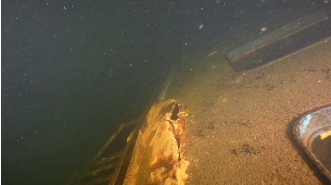
FIG. 3.29: Protrusive deformation on the port side shell plating below Deck 7.
