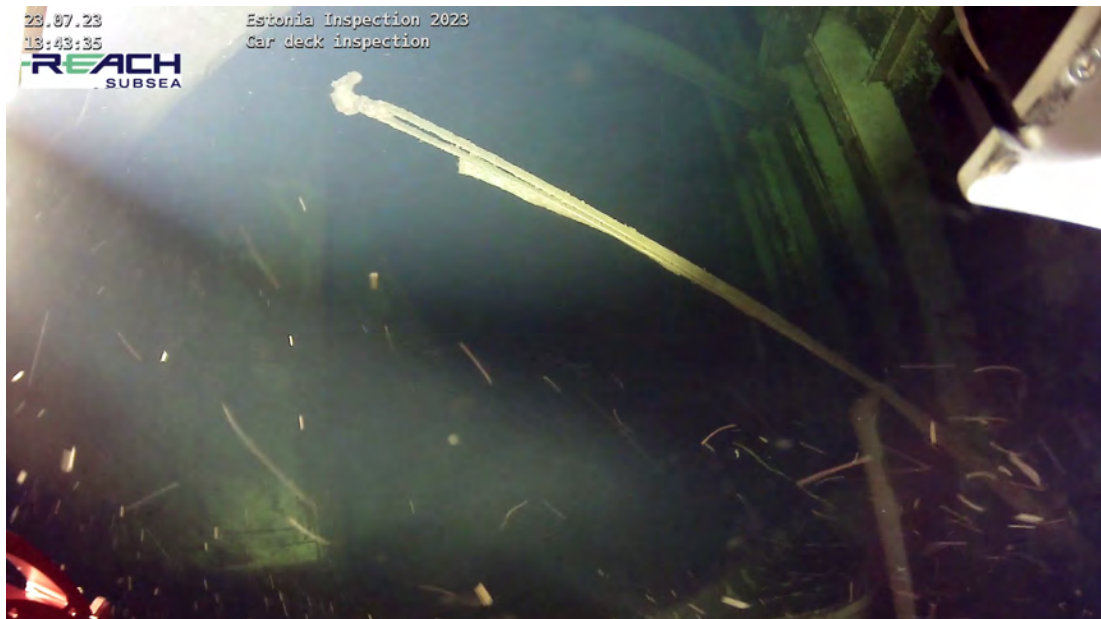
FIG. 5.2: Footage from the car deck shows a disconnected lashing belt from a shifted cargo unit on the car deck of MV ESTONIA during the visual inspection in 2023 (O 2.21).
