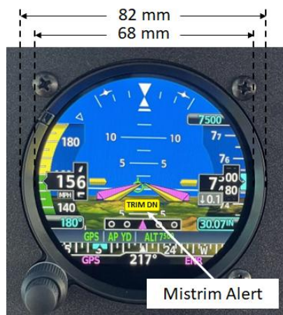
Figure 21. Amber mistrim alert on the PFD indicated by a white arrow. Source: Supercub.org. Annotation and mistrim alert (TRIM DN) added by SHK.
