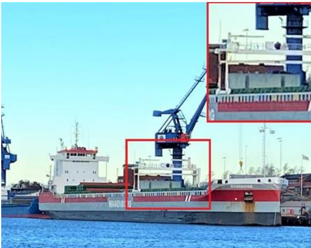
Figure 1. ROERBORG berthed in Oxelösund, but not at the quay where the accident took place. The gantry crane is the white structure visible in the red markings. The blue crane in the background belongs to the port.
