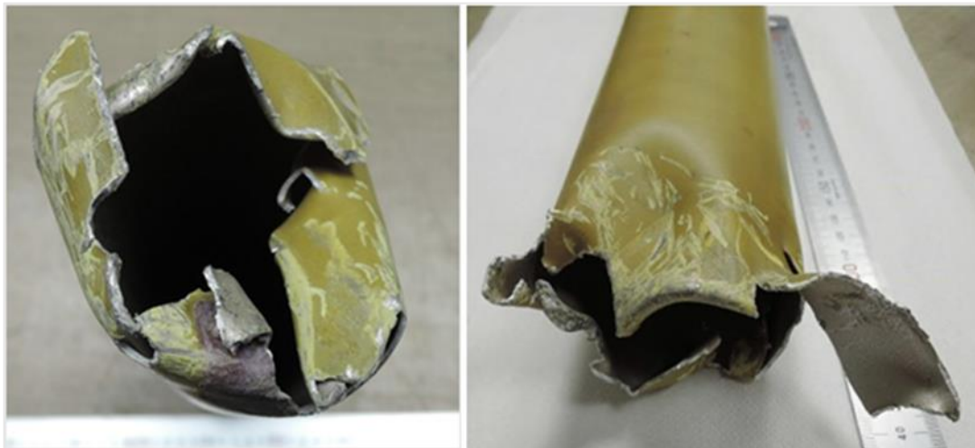
Figure 13. The picture on the left shows the fracture on the section of the drive shaft leading towards the engine. The picture on the right shows the fracture on the section of the drive shaft leading towards the tail rotor gearbox.
