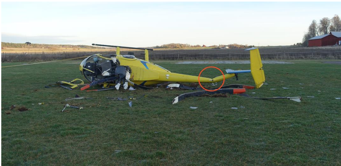
Figure 8. The aircraft wreckage, the damage to the tail boom marked with a circle.
