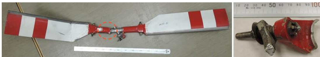
Figure 12. The picture on the left shows the tail rotor, with the marked area indicating the focus of the examination. The picture on the right shows the broken pitch arm along with a section of the pitch link.
