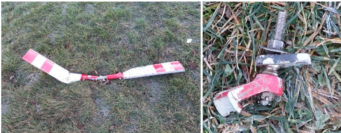
Figure 9. The left image shows the tail rotor where it was found. The right image shows one of the tail rotors blades pitch arms, along with a section of a pitch link.
