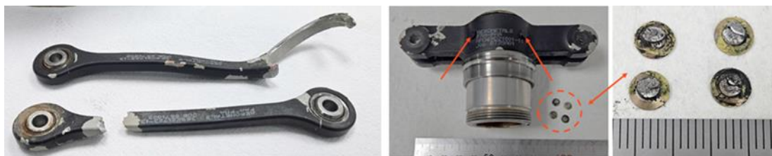
Figure 11. The picture on the left shows the damaged pitch links. The pictures on the right shows the damaged rivets. The rivet heads are coming from the inside of the housing.
