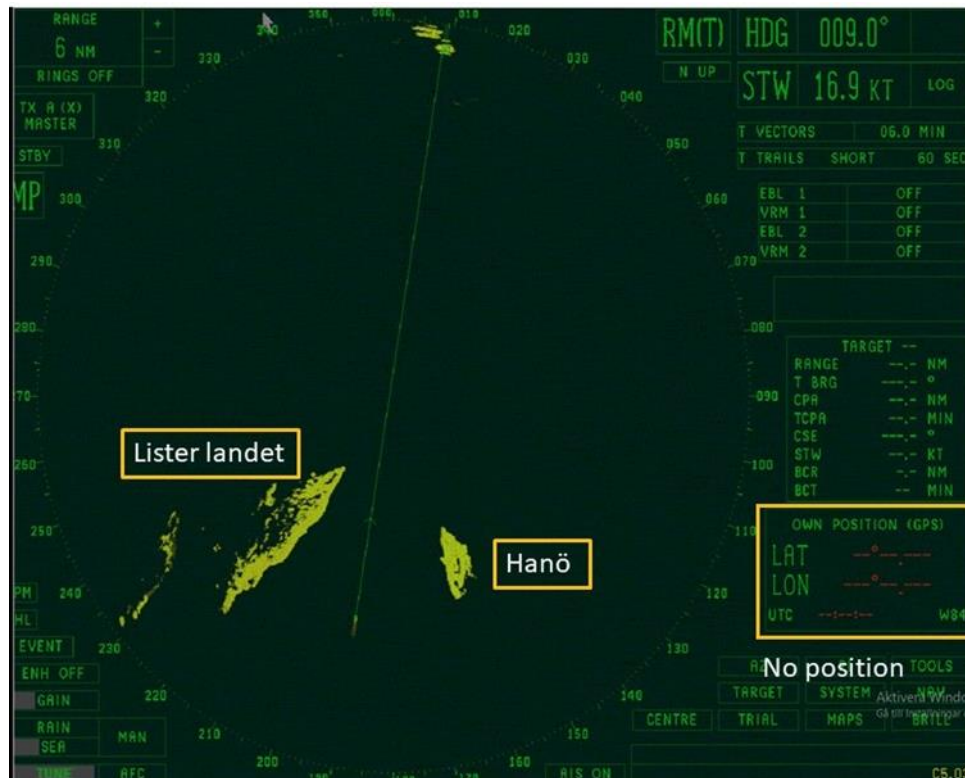
Figure 15. VDR recording of the X-band radar from 05:02 hrs. The yellow fields on either side of the green line showing the course consist of land bodies. Note that no GPS position is presented in the lower right corner (LAT, LON). Boxes and white text inserted by SHK.
