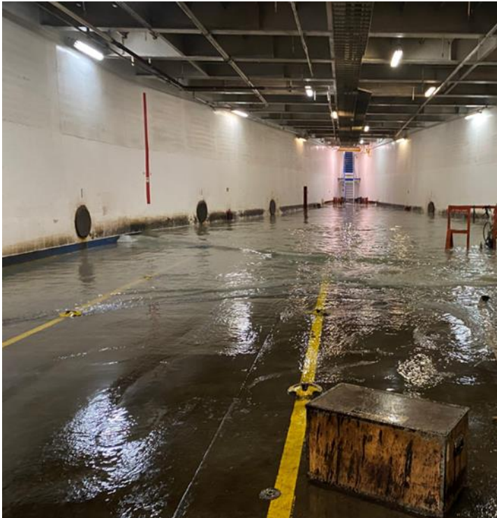
Figure 8. The picture shows water ingress in the lower cargo hold after the third grounding. Picture used with permission of the Swedish Maritime Administration.
