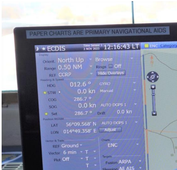
Figure 12. Picture of the ECDIS screen. Photographed during one of SHK's on-board visits after the accident. Note the text on the screen frame on top.
