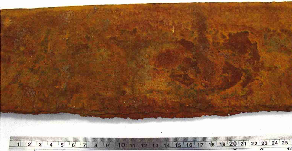
Photo 5. Torn edge of metal strip, view of hull exterior.
