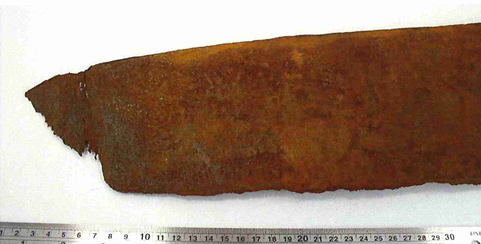
Photo 6. Torn edge of metal strip, view of hull exterior.
