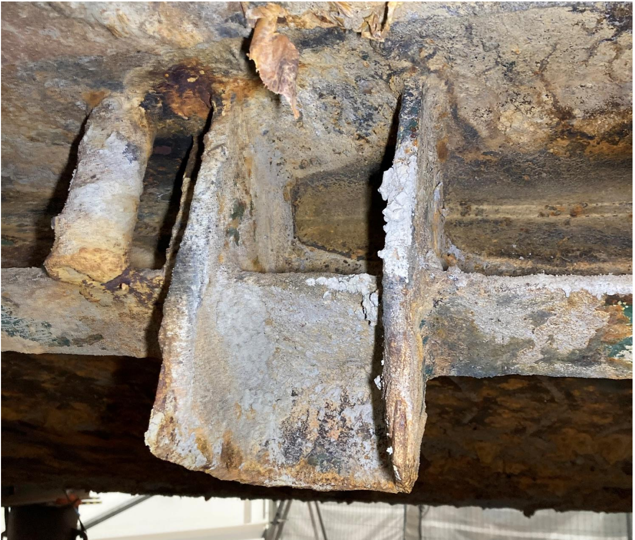
Figure 5. Starboard side upper ramp side lock box.
