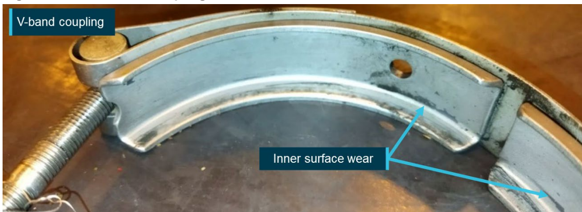
Figure 7: HMU V-band coupling wear location
