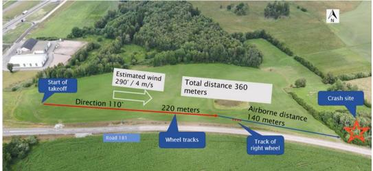
Figure 7. Tracks in the terrain. Markings inserted by SHK. Photo: The Police Authority.
