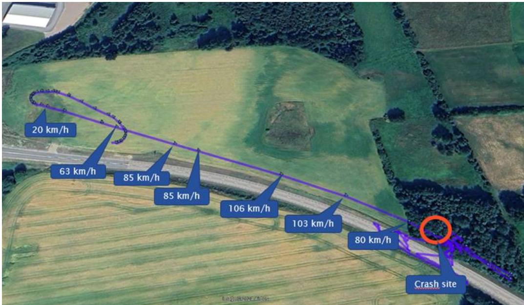
Figure 5. Recorded data from one of the navigation applications with the ground speed. Markings inserted by SHK. Image: Google Earth.
