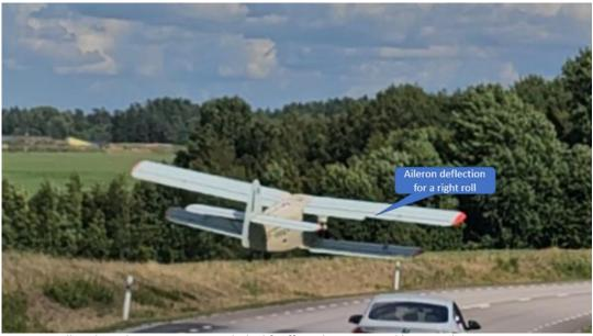
Figure 2. Roll to the right in connection with the lift-off. Markings inserted by SHK. Photo: Private.
