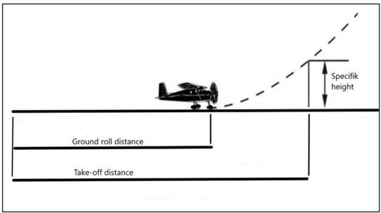
Figur 10. Illustration of ground roll and take-off distances.
