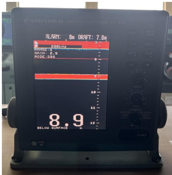
Figure 9. Image of MESHKA's echo sounder. The picture was taken during SHK's onboard visit.
