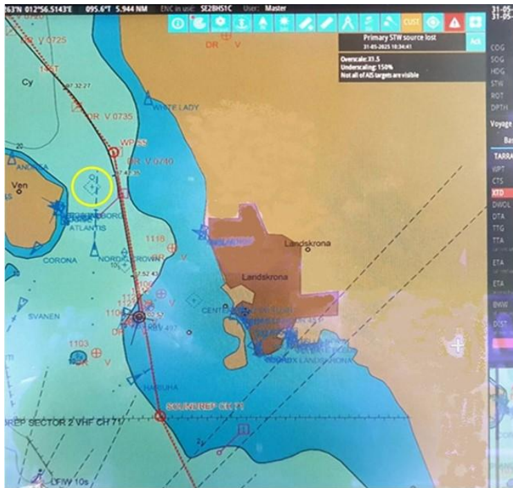
Figure 2. The image shows the chart in MESHKA's ECDIS after the grounding. The ENC is SE2BHS1C, which was the ENC active in the ECDIS system at the time of the grounding. The yellow circle marks the virtual AIS buoy. The image from MESHKA's ECDIS was taken by the Swedish Transport Agency's on-call ship inspector 31 May 2025. The image has been edited by SHK.
