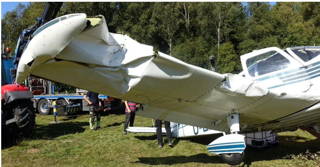
Figure 9. Damages on the right wing.
