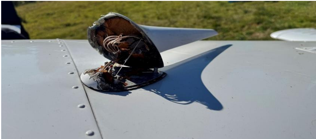
Figure 4. Picture of the damaged communication antenna.
