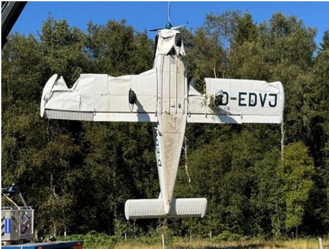
Figure 2. The pictures show the damaged wings and forward part of the fuselage.
