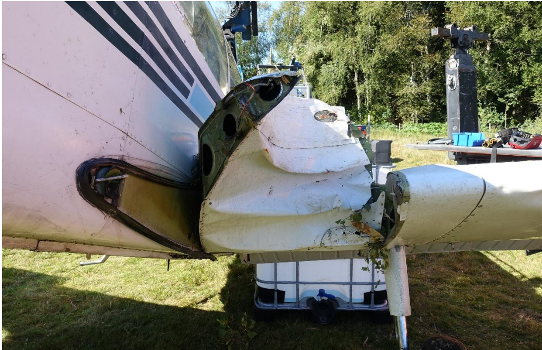
Figure 10. Damages on the left-wing root.
