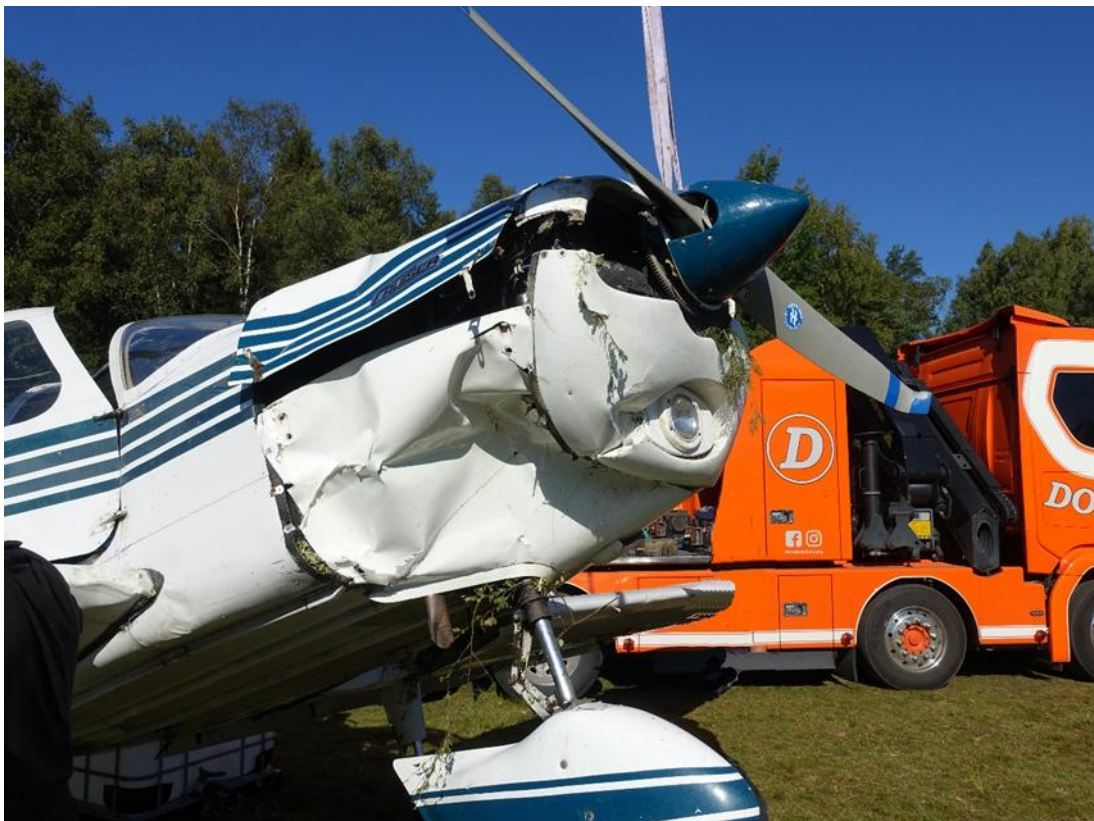
Figure 11. Damages in front of the fire wall.
