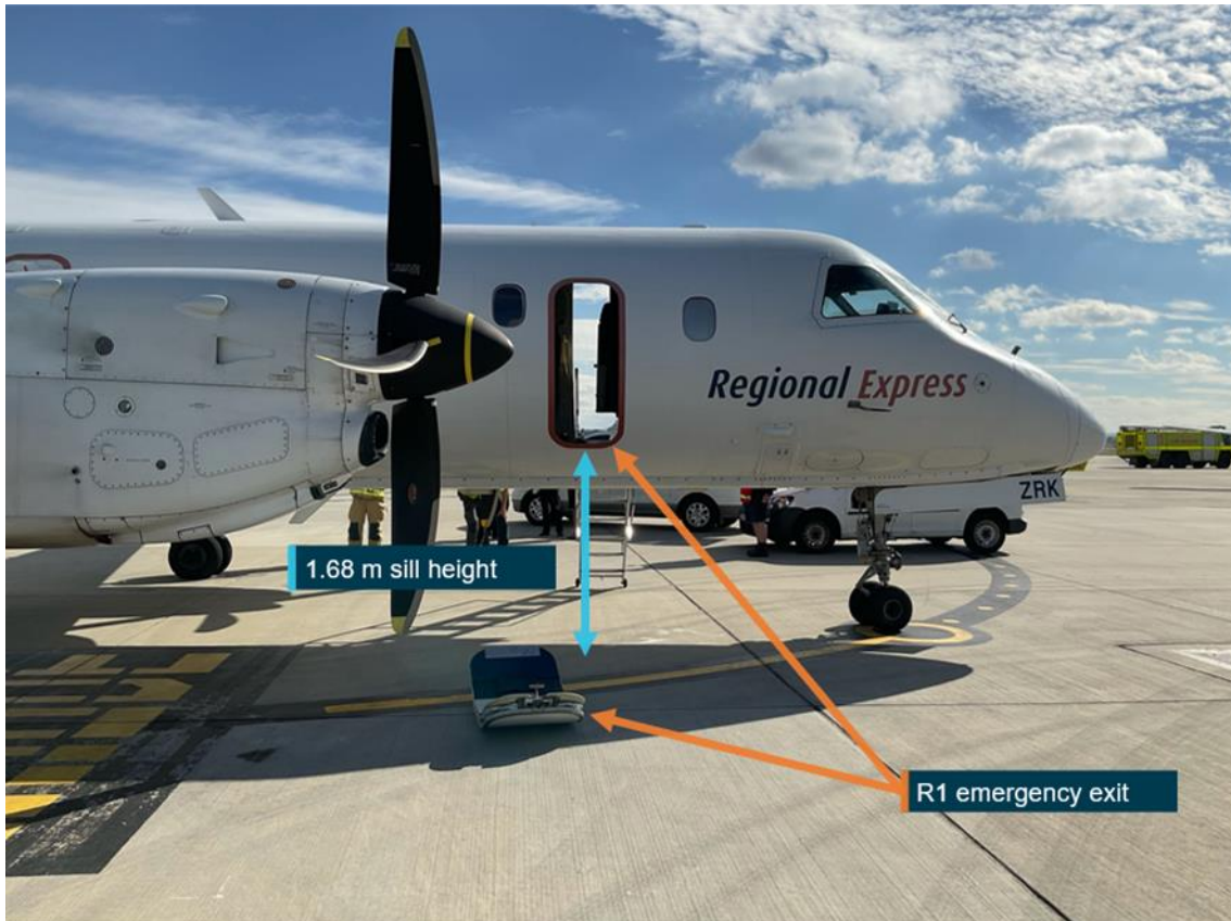
Figure 4: R1 emergency exit on the Saab 340B
