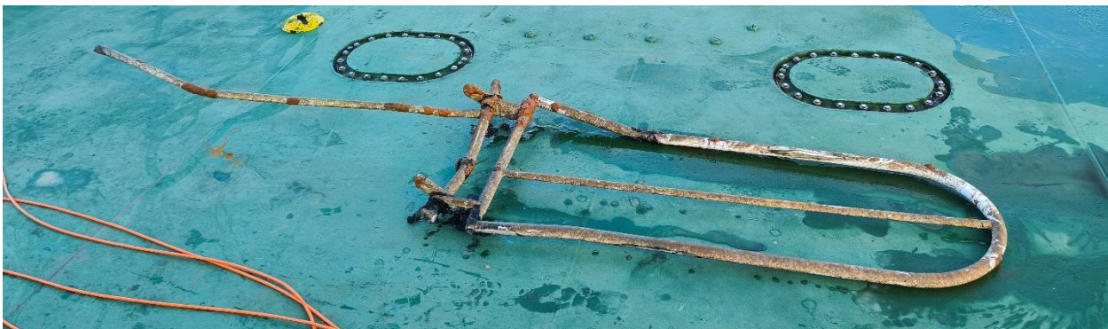
Figure 5. Recovered part of the ramp railing on the aft deck of the survey vessel EVA-316. Source: Tauri Roosipuu, ESIB
