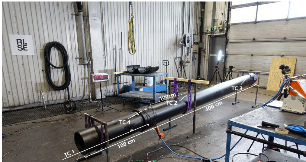
Figure 16. The picture shows the testing arrangement of pipes with the fitted electrofusion coupler. The temperature indicator that was used to register the temperature during the tests are marked in white with the designation TC1-TC4. Source: RISE.
