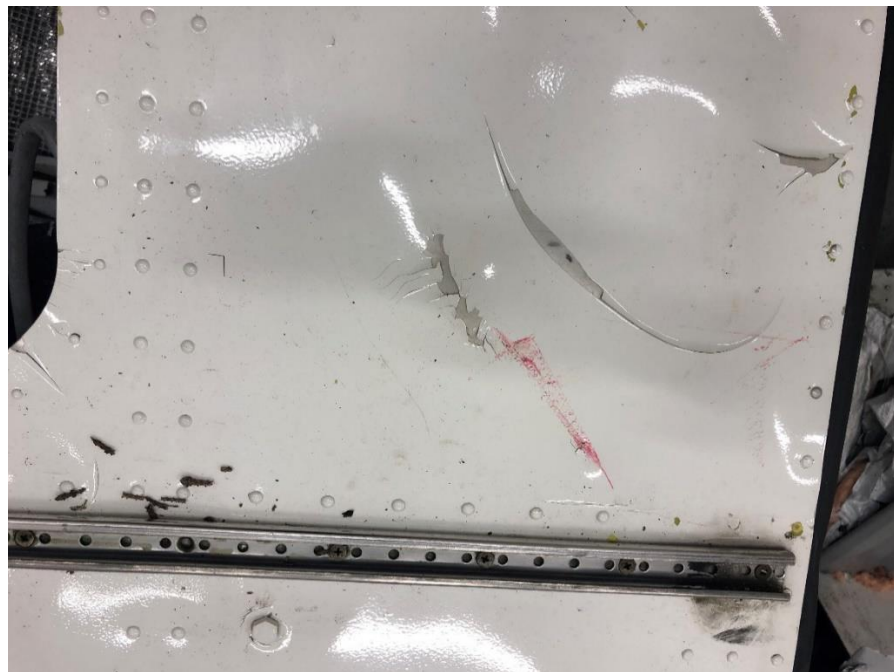
Figure 7. Impact mark from the door handle on the fuselage of SE-MES.
