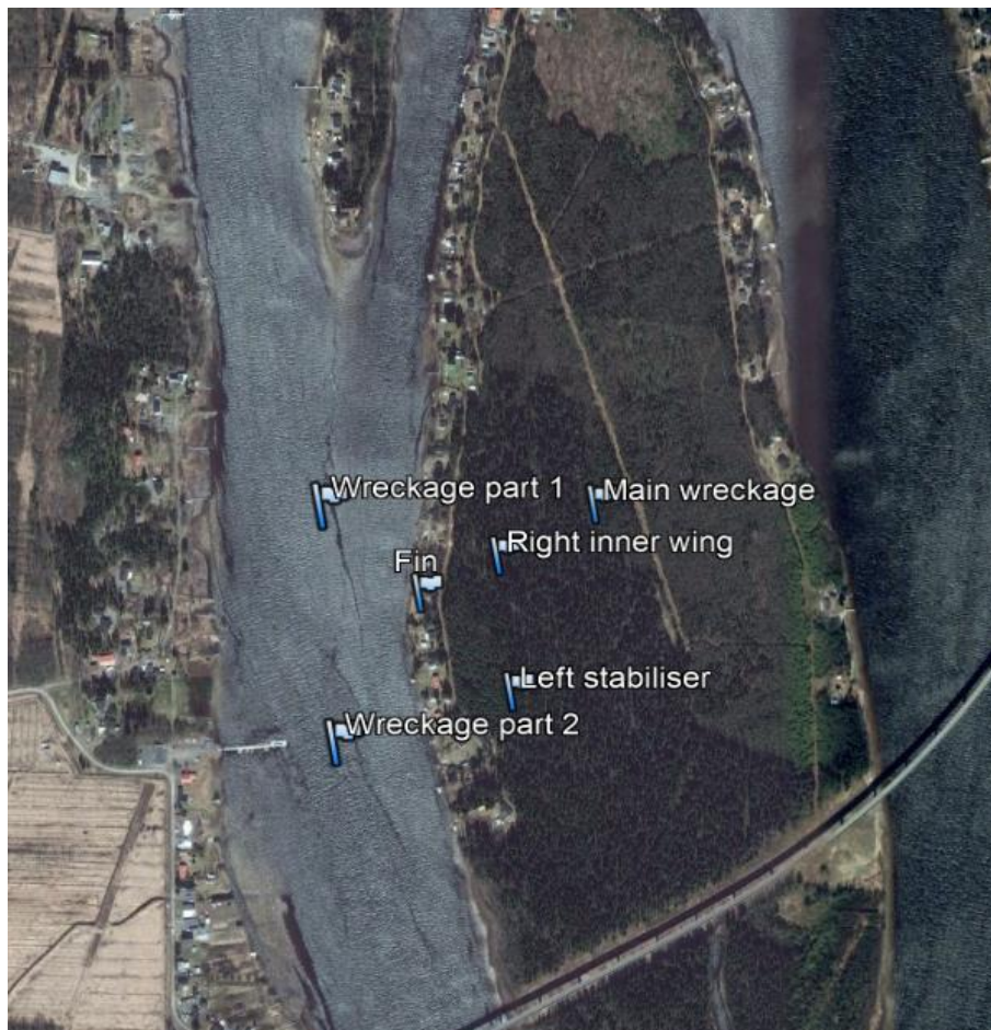
Figure 5. Site of the accident and location of the parts of the wreckage. Photo: Google Earth: © Lantmäteriet Ref. R61749_190001.
