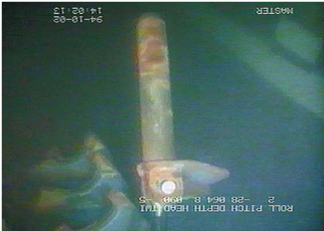
FIG. B.3: The locking bolt for the bottom lock, filmed on the wreck. The bolt was salvaged and examined by investigators, but was not saved. To the left bottom of the picture, the remains from the three broken attachment lugs are seen. The image is from the JAIC report, Figure 8.15, and is turned upside-down (to compensate for the vessel lying effectively upside-down when filmed).
