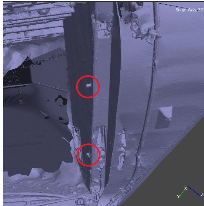
FIG. B.2: An image from the photogrammetry acquired in 2022. The lower red circle displays the same locking as Figure B.1, i.e., the port side lower bow ramp locking.
