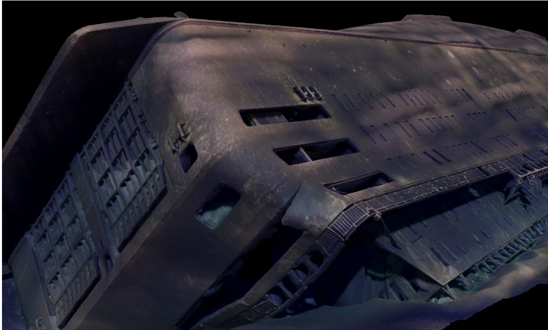
FIG. 3.2: Port side stern of MV ESTONIA, showing a crack on deck 6. From the crack, the vessel is twisted along deck 6 and forward. Image from photogrammetry.
