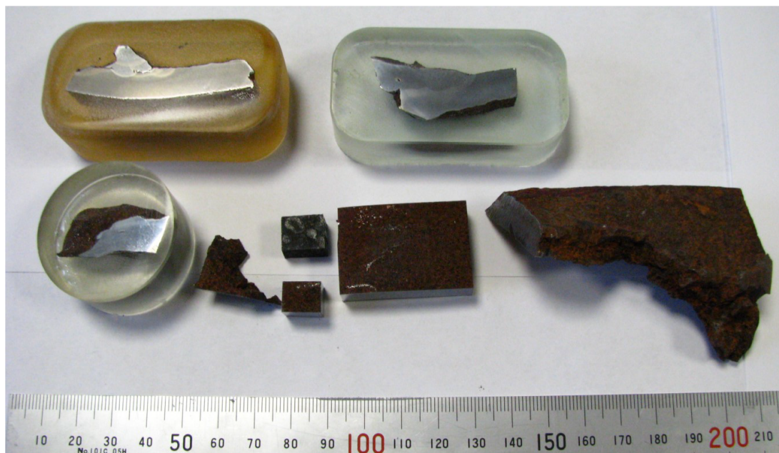
FIG. 3.4: Samples from the bow visor, subject of examination by Norwegian University of Science and Technology as well as Element Material Technology AB. Photo: Element Material Technology AB.
