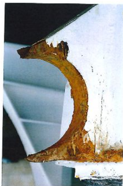
Figure 8.22 Failed port lug of visor port hinge.
