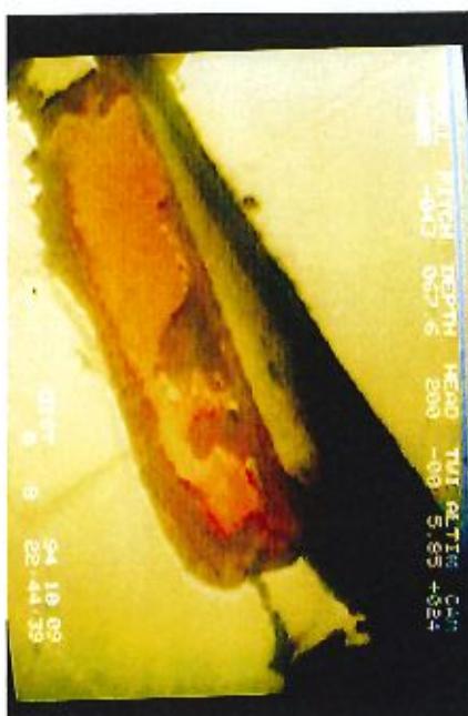
Figure 8.18 Bottom face of the starboard side locking lug.
