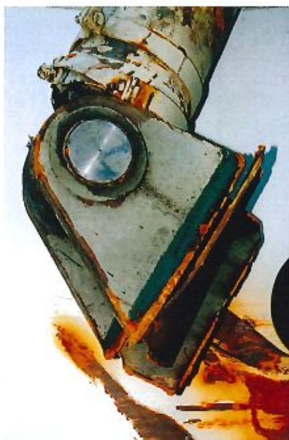
Figure 8.26 The bottom end of the visor port side opening actuator.
