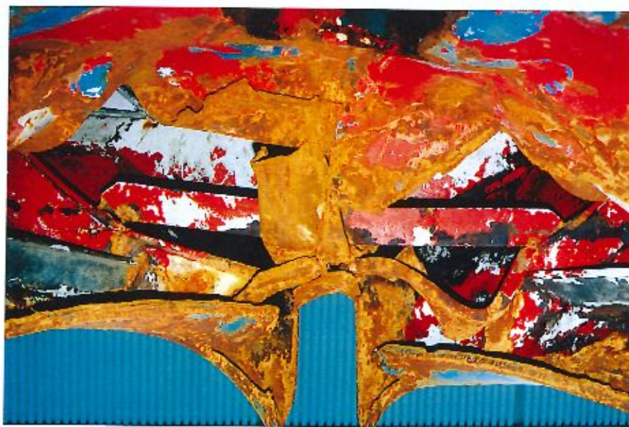
Figure 8.6 Damage to the bottom structure of the visor.
