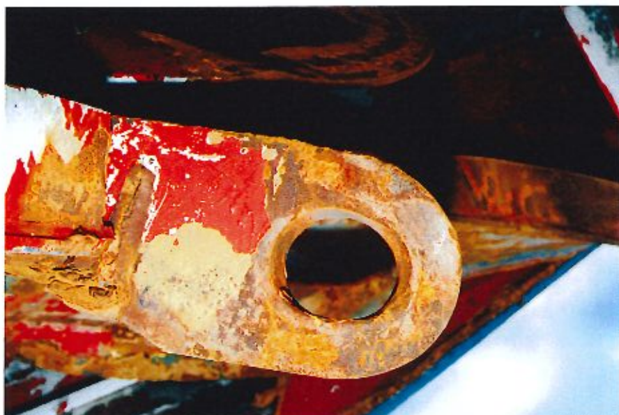
Figure 8.10 The visor lug for the bottom lock.
