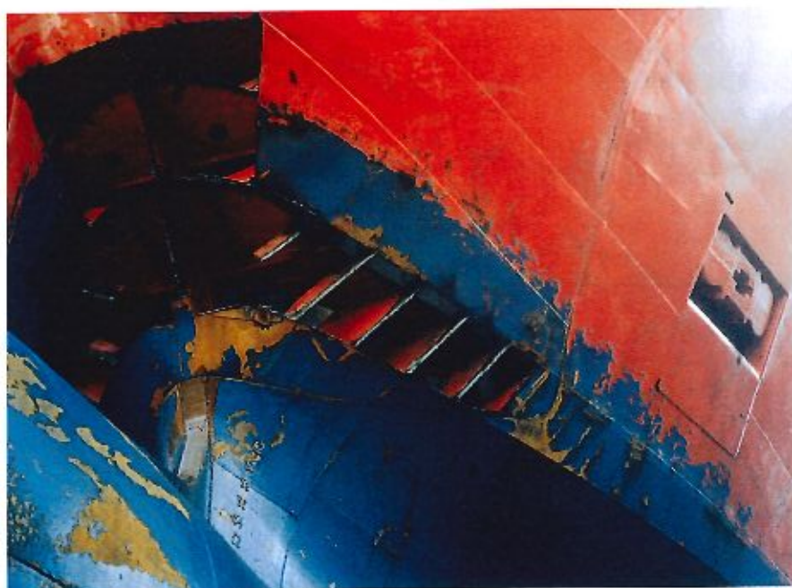
Figure 3.12 The extent of ice damage repair in 1987.
