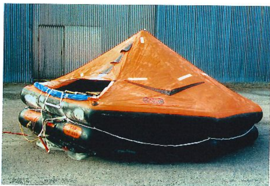
Figure 17.7 ESTONIA's Viking 25-K type liferaft.
